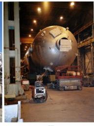
In most cases the plant equipment is not designed to perform such a close temperature control during inital start-up. But creates a rather radiant heating with a non-uniform heat distribution.
