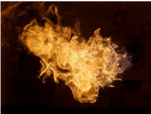
FIGURE 2 - QUADRAFLO Conical at 1.0 MW, natural gas and oxygen, low momentum setting.
