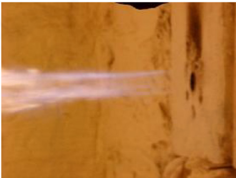
FIGURE 4 - QUADRAFLO Conical hot face view at 1.0 MW, natural gas and oxygen, low momentum setting.
