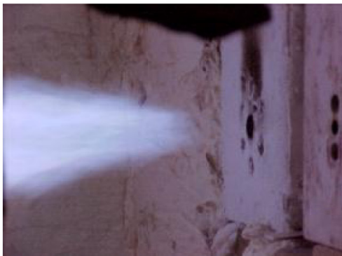
FIGURE 3 - QUADRAFLO Conical hot face view at 1.0 MW, natural gas and oxygen, high momentum setting.
