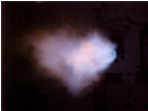
FIGURE 1 - QUADRAFLO Conical at 1.0 MW, natural gas and oxygen, high momentum setting.
