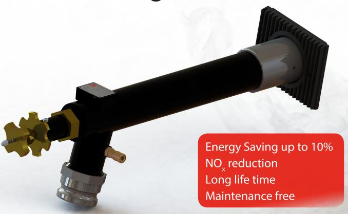
Hotwork Internationals Underport and Sideport Burner systems incorporate burner sealing plates, which eliminate the inclusion of tertiary air. Gas (RGB) and Oil (ROB) Burners are equipped with ball end nozzles which fit into the ribbed socket of the sealing plates. This gives good heat resistance and a simple tight seal. Burner nozzles are made of special nickel free high temperature resistant steel, giving long life time.
