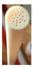
Material: High Temp. Resistant Ceramic Temperature: Up to 1900°C Dimensions: Diameter 15mm, length 1500mm (standard) extended version up to 2000mm Upgrade: Platin coating
